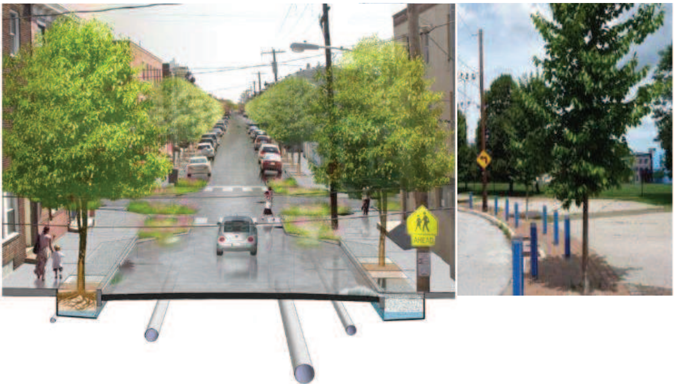
Fig. 4.3 Árboles-trinchera (Philadelphia water department, 2011).
